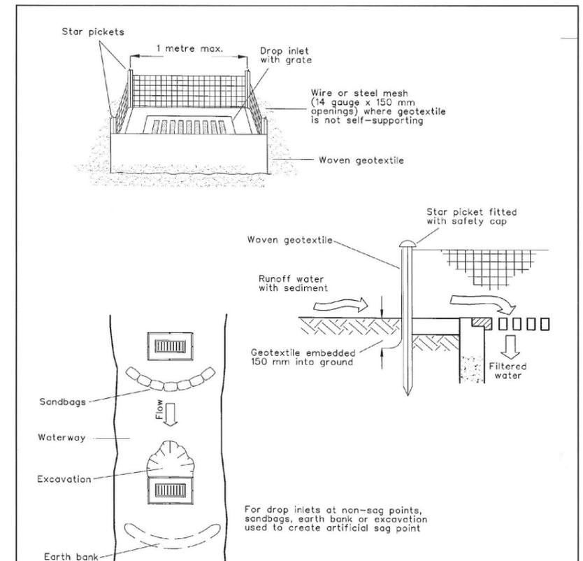
For drop inlets at non-sag points, sandbags, earth bank or excavation used to create artificial sag point
